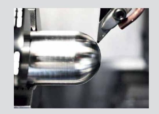
PCBN and PCD are high-performance tool material from a polycrystalline mass, produced in high temperature-pressure process.
