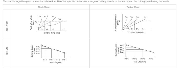
This double logarithm graph shows the relative tool life of the specified wear over a range of cutting speeds on the X-axis, and the cutting speed along the Y-axis.
